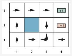
Two optimal policies for the grid environment, stating which actions to do in each state.
